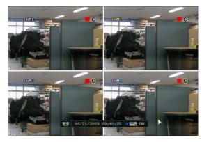
2 different display modes are supported by the 4 channel DVR. By repeatedly pressing the **DISPLAY** button, the operator can choose between single screen, 4 screen and basic sequence modes.
