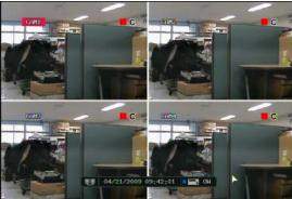
Press the Enter button. Then red square on camera title will be shown. If pressing the Enter button again by moving the navigation key, user can select the single display channel.
