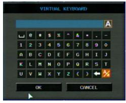
After startup diagnostics are complete, the operator must logon to the system. The default user name is 'ADMIN'. the default password of '1234' and press the **ENTER** button.
