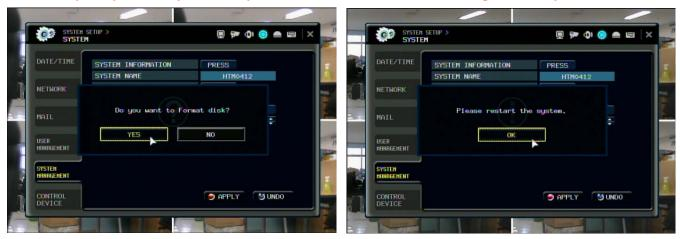
SYSTEM DATA : System settings can be saved to a USB memory stick. The settings can be reloaded in case of accidental factory reset or can be transferred to another DVR if multiple units need to be installed with the same settings. After loading the configuration data, system will be rebooted
