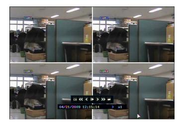
By pressing **DISPLAY** or using the **CHANNEL SELECTION** buttons, it is possible to display a single screen or 4 screens in a similar way to the live display mode.
