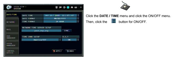
**DATE TIME** : Allows the operator to set or modify the current date & time.
